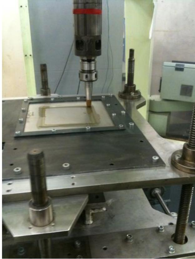
**Fig. 1.** Asymmetric Incremental Sheet Forming (AISF), the work piece is clamped in position while the tool head “pushes out” the desired shape, on release springback occurs as a result of which the final shape is not the desired shape
