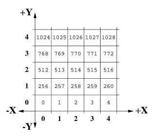
Figure 1. Addressing for 2D 5x5 object space
