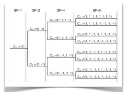
These codes are derived from an OVSF code tree, and each user is given a different, unique code. An OVSF code tree is a complete binary tree that reflects the construction of Hadamard matrices.
