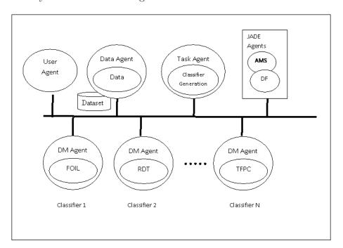
Figure 7.1: Classifier Generation EMADS Model Architecture
