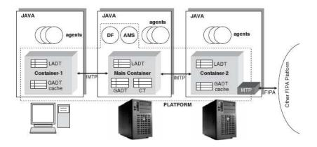
Figure 3.4: JADE Architecture (Bellifemine et al., 2007) [16]
