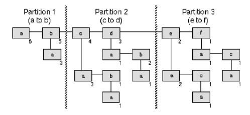
Figure 6.1: Vertical Partitioning of a T-tree Example [29]
