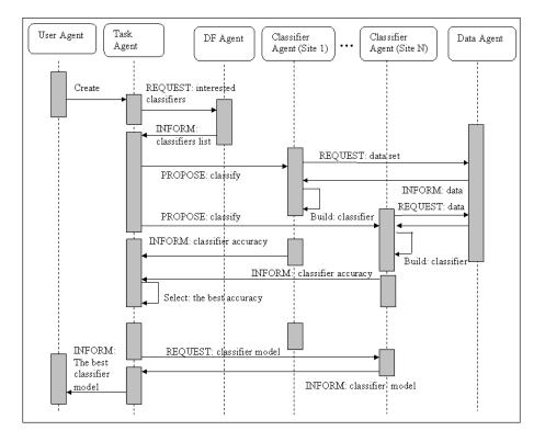
Figure 7.2: Classification Task Sequence Diagram.
