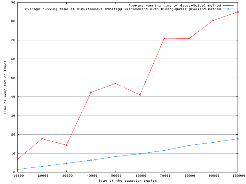
Fig. 1. The blue line shows the average successful running time of simultaneous strategy improvement that uses Biconjugated gradient method as its sparse linear solver. The red line is the average running time of the Gauss-Seidel method.
