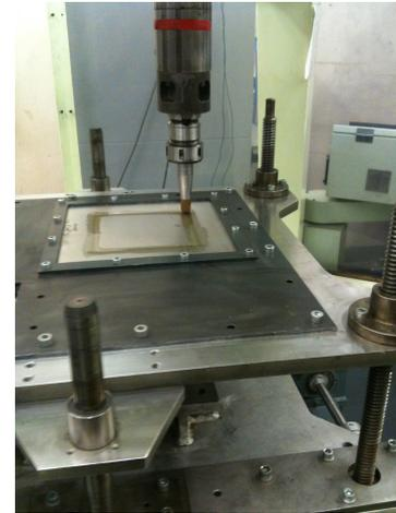
FIGURE 3.2: Example AISF machine 2, a metal sheet is clamped into a holder and the desired shape is produced using the continuous movement of a simple round-headed forming tool.
