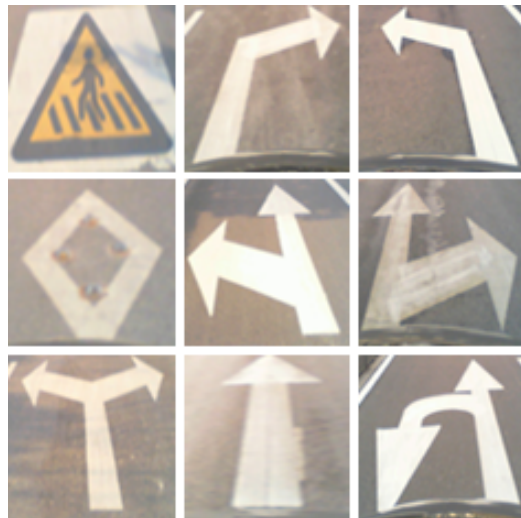
Fig. 2. Illustration of road surface traffic signs
