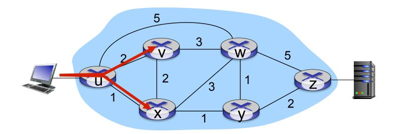
Q: what if network operator wants to split u-to-z traffic along uvwz and uxyz (load balancing)?
