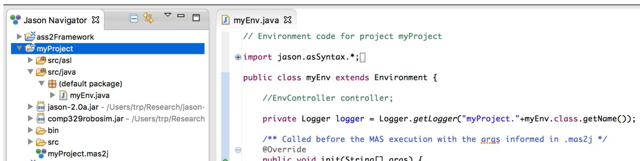
You will need to create a new object of the **EnvController** class, which configures the simulator. You can also request from this object a reference to **RobotMonitor** Object, which will provide you control of your robot.
